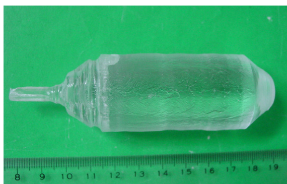
Figure 1. Photograph of 10 at.% Yb:GSO crystal grown by Czochralski process.
